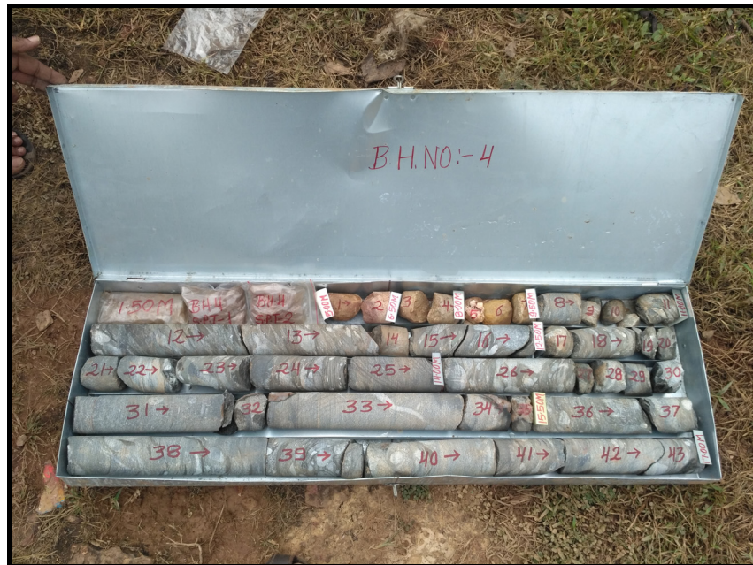
SOIL/ ROCK SAMPLES COLLECTED FROM TRIAL BORE
