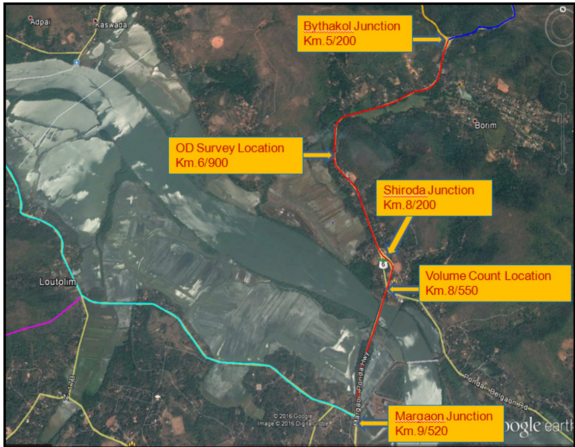
Figure 5.2 Traffic Survey Locations
