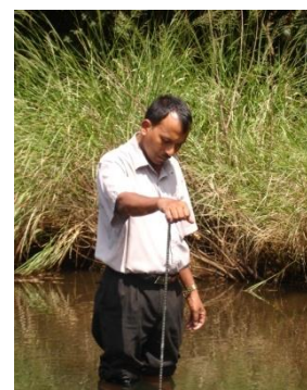
Using pygmy current meter to measure flow
